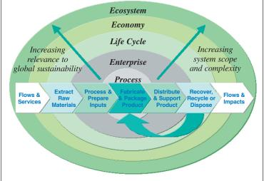
Figure 1. Hierarchy of sustainable process systems engineering. Each successive oval encompasses a broader set of life cycle steps. Gray areas represent existing PSE techniques. Green ovals represent new frontiers for PSE.
